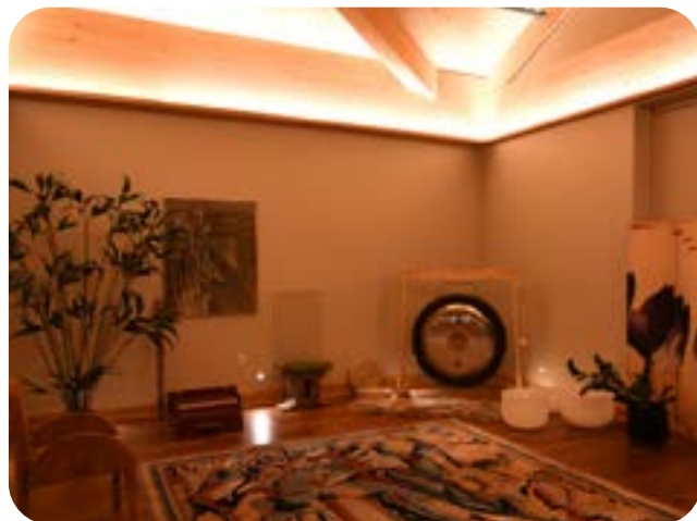
T3 emphasizes mass timber roof while providing soft indirect light. Fully dimmable floor and ceiling set mood. Sliding wall is closed to block out window.
