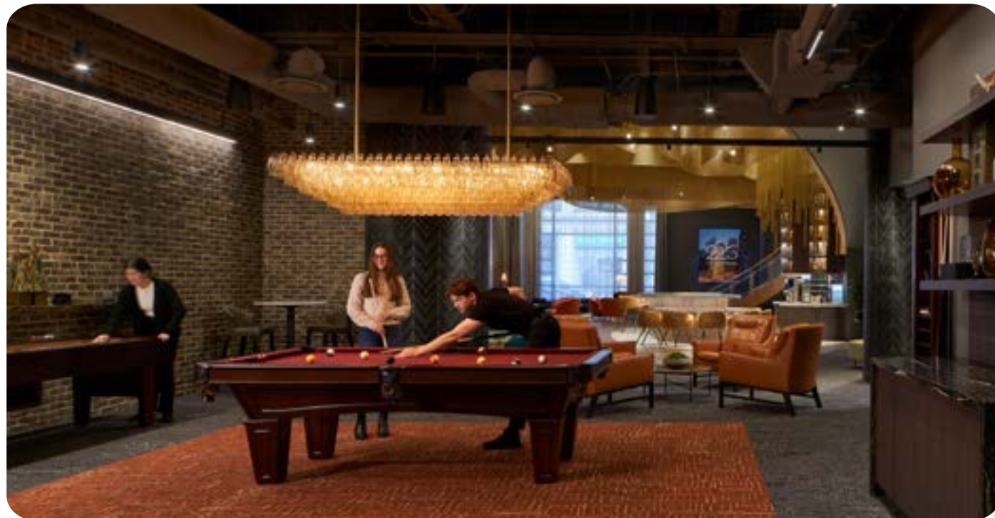
The first look at the amenity bar/lounge reveals the scrim curtain chandelier, grazing light at the back wall, and main bar accents, adding depth (above). Maintaining the warm, residential feel, the lower-level gaming showcases vertical brick grazing and a pool table luminaire, both highlighting and focusing attention on this amenity (below).
