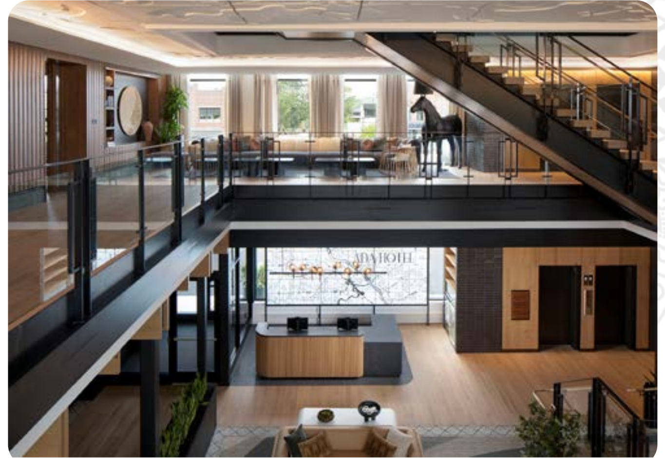
Second floor event and gathering space utilizes miniature track spotlights while low profile LED tape with graze optic provides ambient lighting throughout the atrium (above). The intimate lounge within the third-floor bar achieves a delicate balance of natural light and nostalgic illumination, creating a warm and inviting atmosphere (below).
