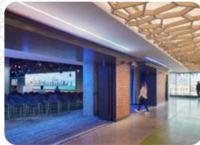
The color changing linear wallwash fixtures can be controlled by the main room's production systems to signal guests when an event is about to begin.
