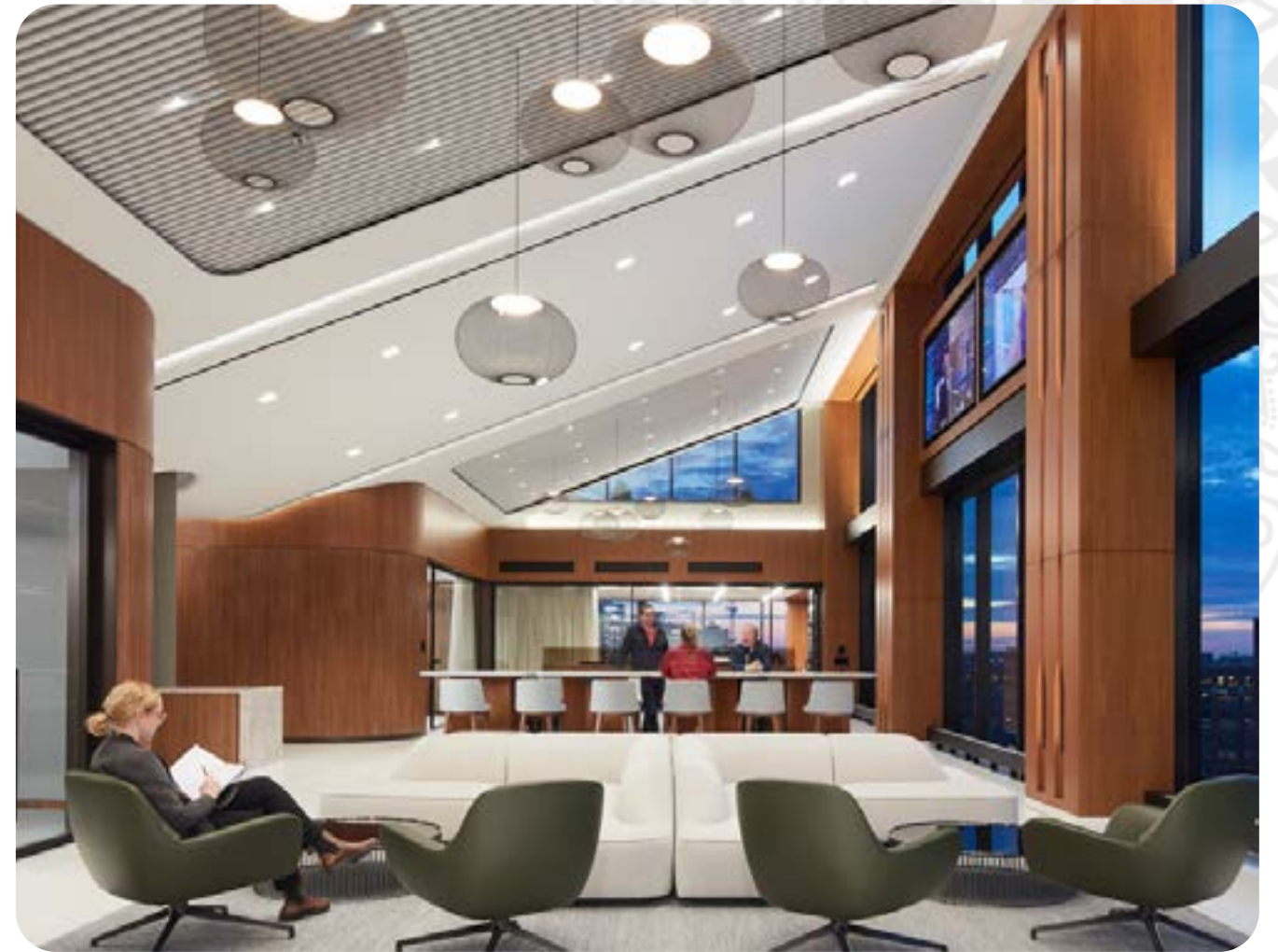
Elements work in harmony. Uplight at outer bays segment room without obscuring screens. Millwork column light detail acts as destination marker from entry (above). Linear lensed slot elements trace curved ceiling lines, guiding visitors from the entrance to the expansive huddle space. Miniature downlights provide general lighting (below).
