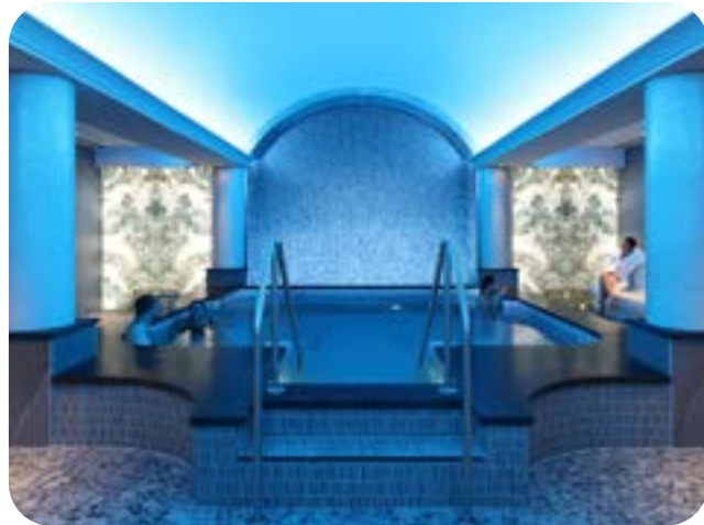
Hydro-therapy light immersion creates a mood. Preprogrammed shows adjust color sequences for central vault, side coves, and pool lighting while balancing white lighting elements.
