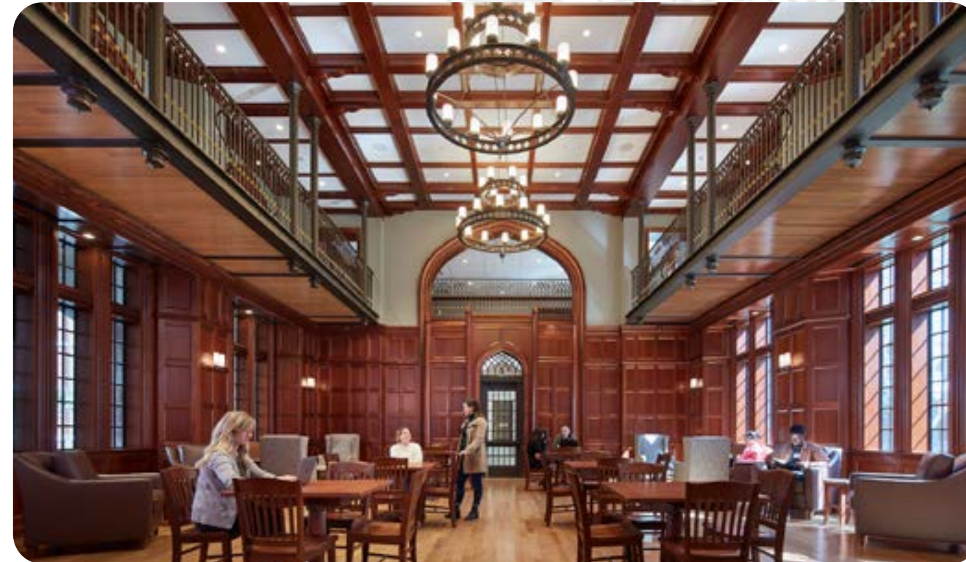
The Rothschild Great Room utilizes two-tier chandeliers with cylindrical diffusers, companion wall sconces, and recessed downlights for reading tasks (above). The Carmichael Dining Hall features custom chandeliers with glowing globes and concealed uplight rings, custom sconces, and recessed downlights, all separately controlled for layered illumination (below).
