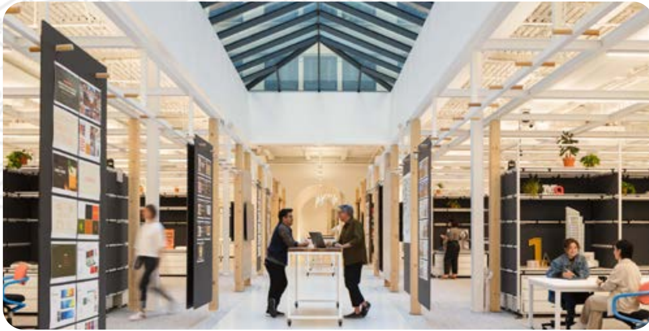
The “Hall” is a bright, collaboration area. Concealed uplights above trellis beams and linear, lensed downlights below illuminate desks and provide balance with daylight (above). Direct-indirect cylinders celebrate the “Solarium’s” tall ceilings, large-scale pendants illuminate the plant-filled counters, and “grazers” highlight pilasters to balance contrast with daylight windows (below).
