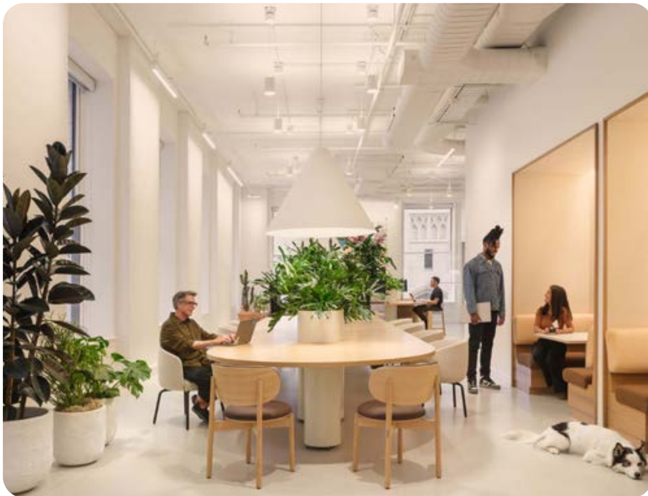
The “Hall” is a bright, collaboration area. Concealed uplights above trellis beams and linear, lensed downlights below illuminate desks and provide balance with daylight (above). Direct-indirect cylinders celebrate the “Solarium’s” tall ceilings, large-scale pendants illuminate the plant-filled counters, and “grazers” highlight pilasters to balance contrast with daylight windows (below).
