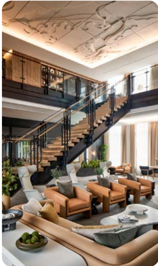
Daylight from clerestory windows, indirect electric light above the wood structure, and vintage-inspired luminaires seamlessly balance transitions between day and night (above). 3D topographic map of the surrounding riverbed is highlighted with perimeter graze lighting while providing volumetric illumination to the lobby for a dynamic visual effect (below).
