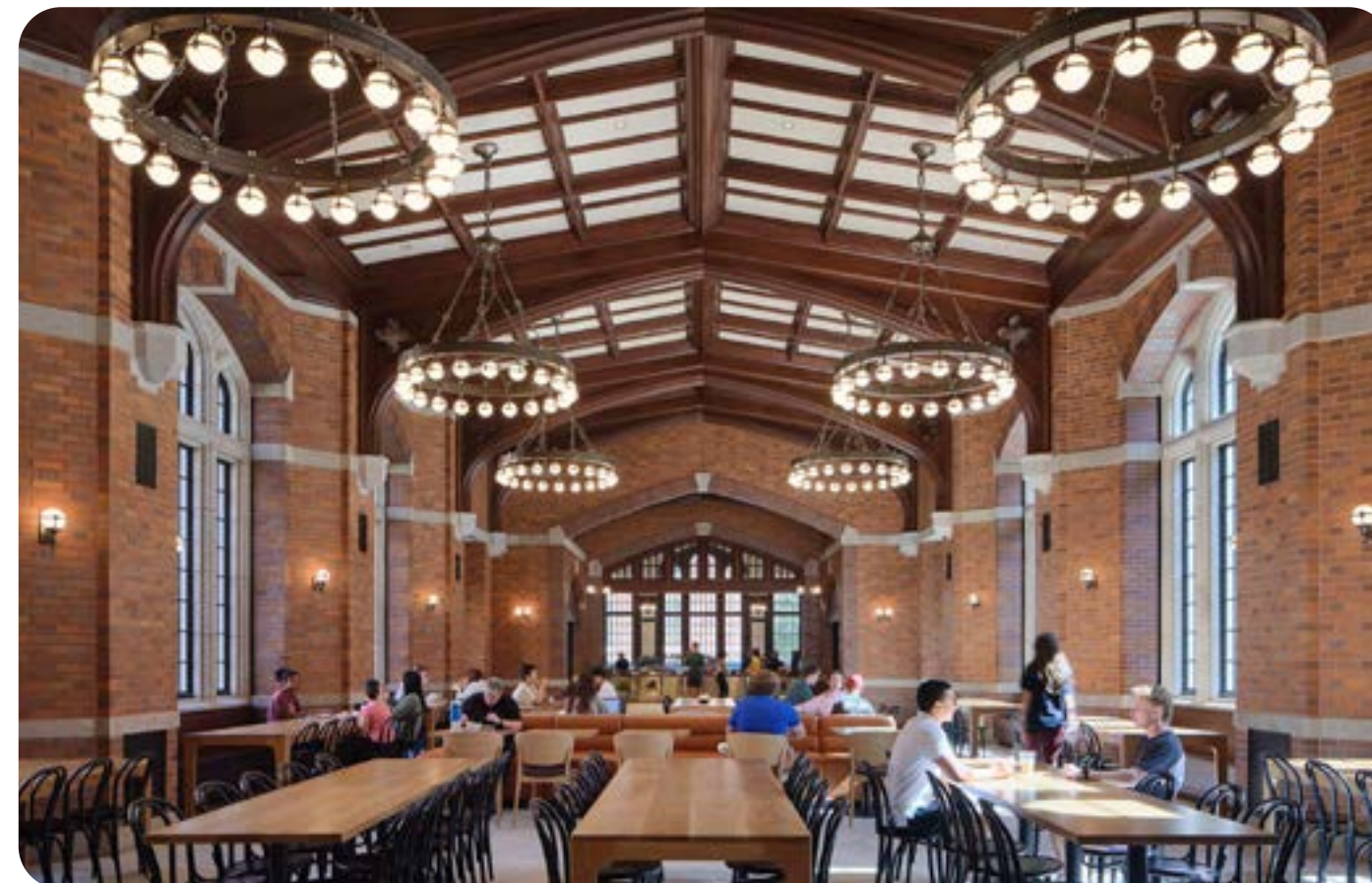
The Rothschild Great Room utilizes two-tier chandeliers with cylindrical diffusers, companion wall sconces, and recessed downlights for reading tasks (above). The Carmichael Dining Hall features custom chandeliers with glowing globes and concealed uplight rings, custom sconces, and recessed downlights, all separately controlled for layered illumination (below).
