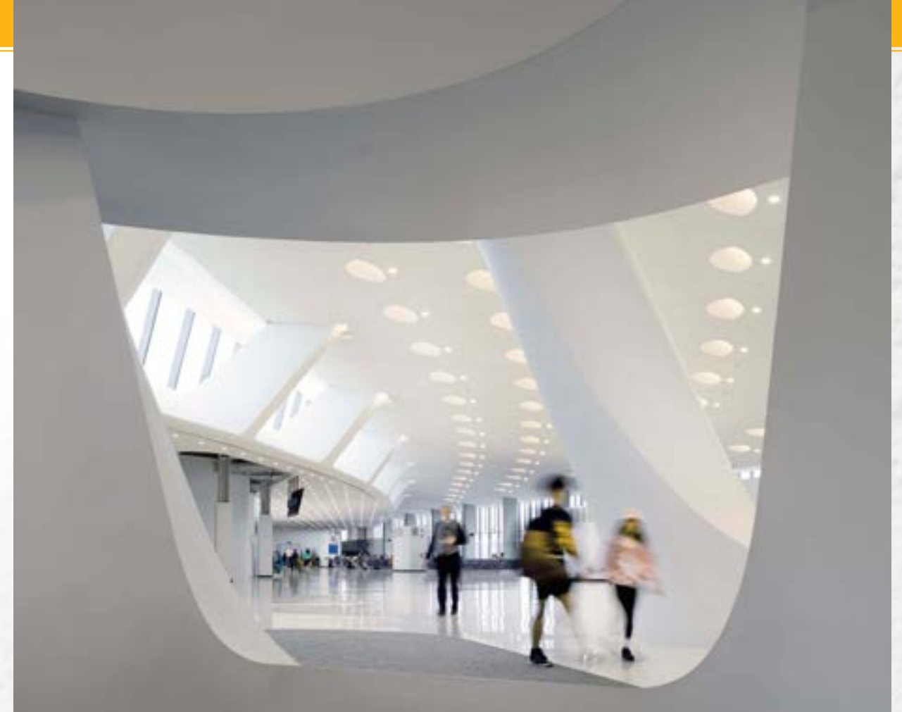
The urban plaza-inspired terminal, exhibiting its twisting columns and "eyelid-shaped" domes. Uniformly illuminated domes are fitted with a single, 2-foot asymmetrical uplight with 3000K CCT.
