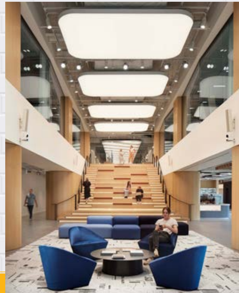
A large skylight above the geometric grand stair seamlessly integrates natural with artificial light. Warm CCT, small-aperture downlights recessed into warm-wood soffits supplement natural light.
