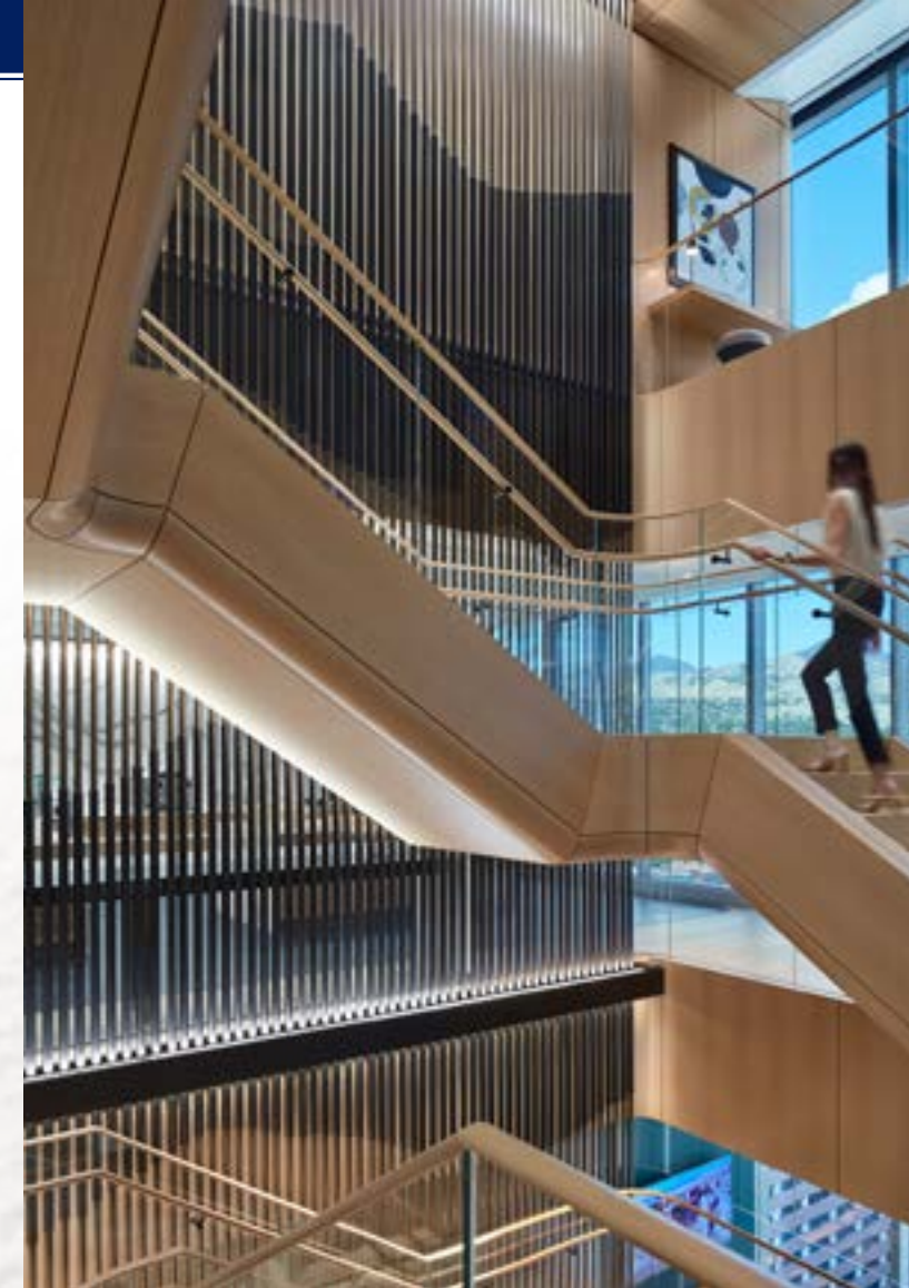
Grazers are concealed behind architectural fascias that are in front of the vertical rods. Integration, output, distribution, glare control, and color temperature were key considerations.
