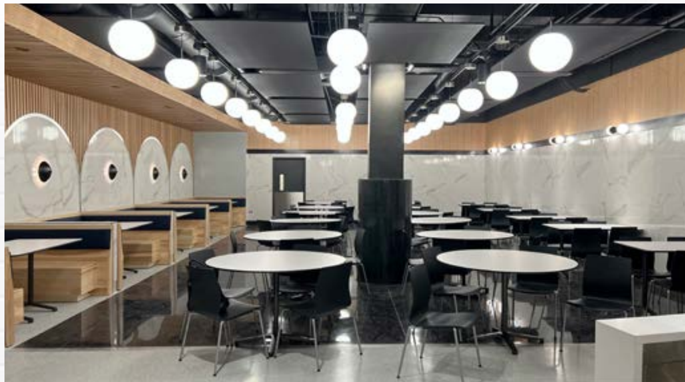
Glowing pendants provide general illumination to the south dining rooms, supplemented by integrated downlights above booths and cylinder downlights concealed above acoustic panels.
